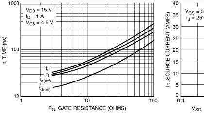
Figure 9. Resistive Switching Time Variation vs. Gate Resistance
