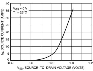
Figure 10. Diode Forward Voltage vs. Current
