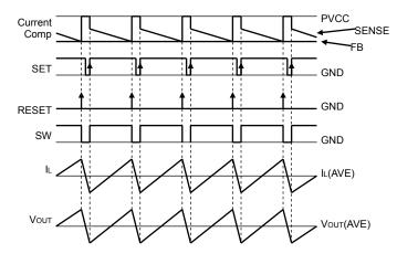
Fig.20 PWM switching timing chart
