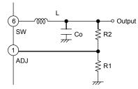
Fig.34 Determination of output voltage
