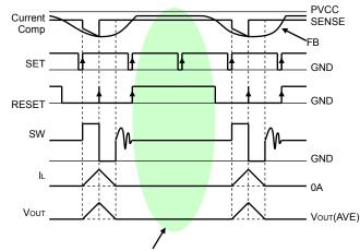
Not switching Fig.21 SLLM<sup>TM</sup> switching timing chart
