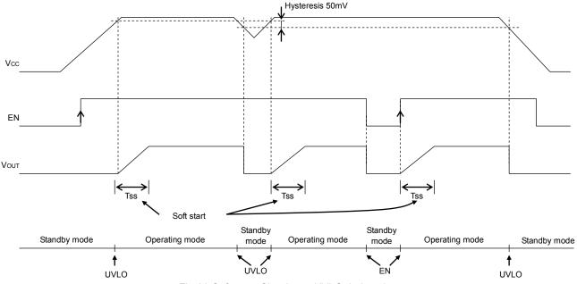
Fig.22 Soft start, Shutdown, UVLO timing chart
