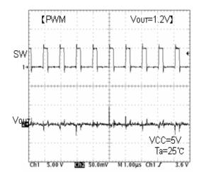
Fig.16 SW waveform Io=3A
