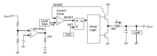
Fig.19 Diagram of current mode PWM control
