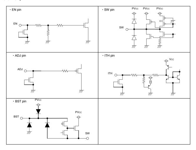
Fig.37 I/O equivalence circuit
