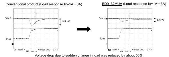
Fig.24 Comparison of transient response
