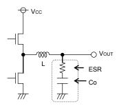
Fig.29 Output capacitor
