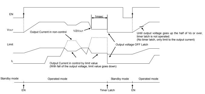
Fig.23 Short-current protection circuit with time delay timing chart
