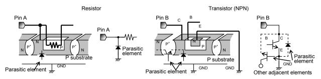
Fig.38 Simplified structure of monorisic IC
