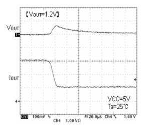
Fig.18 Transient Response Io=3→1A (10  $\mu$  s)
