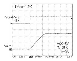
Fig.14 Soft start waveform
