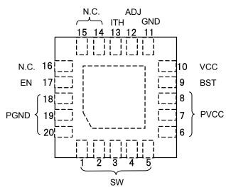
Fig.2 Pin Configuration
