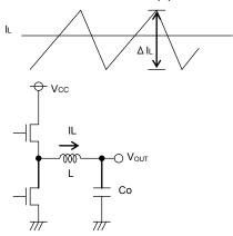
Fig.28 Output ripple current
