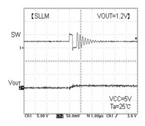
Fig.15 SW waveform lo=10mA
