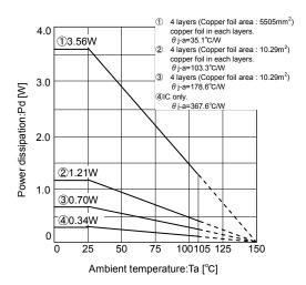
Fig.27 Thermal derating curve (VQFN020V4040)
