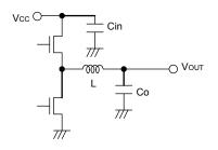
Fig.30 Input capacitor
